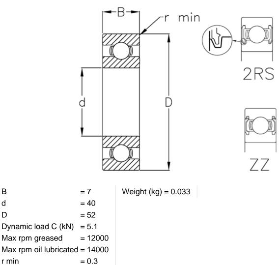
Static load C0 (kN) = 4.4
